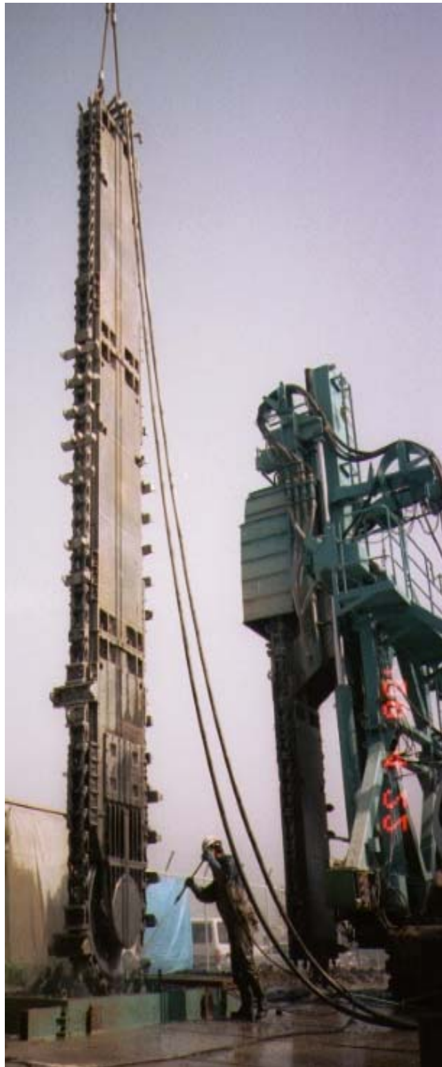
Figure 8. TRD “Cutting Post,” showing the cutting chain. (TRD promotional information.)
